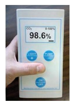
The **GD-888 SERIES** is a family of Infrared Carbon Dioxide gas analyzers that use the latest state-of-the art non-dispersive infrared technology. Rechargeable batteries allow for several hours of portable operation between charges. The GD-888 SERIES puts CO<sub>2</sub> detection in the palm of your hand.
