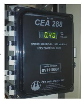
The **CEA 288** is a wall mounted continuous non-dispersive infrared (NDIR) Carbon Dioxide (CO<sub>2</sub>) analyzer contained in a water resistant, dust tight NEMA 4X enclosure. Standard ranges are 0-10,000 ppm (0-1%), 0-10%, or 0-100%. Other ranges are available including 0-2000 ppm, 0-5000 ppm, 0-2%, 0-5%, 0-20%, 0-50% and more.
