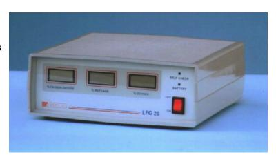
The **LFG 20 PLUS** permits simple and precise measurements of Carbon Dioxide (CO2), Methane (CH4), and Oxygen (O2) in a sample drawn by an internal pump at 200 mL per minute.
